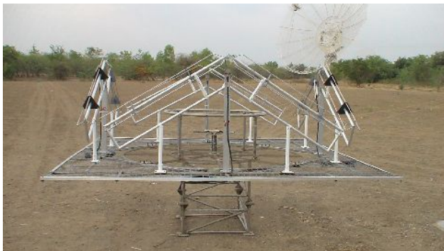
Fig. 3. Low Frequency Feed in boxing ring configuration co-located with the existing 327 MHz GMRT feed with extended reflector. The picture to the right shows its mounting on the turret of a GMRT antenna.
