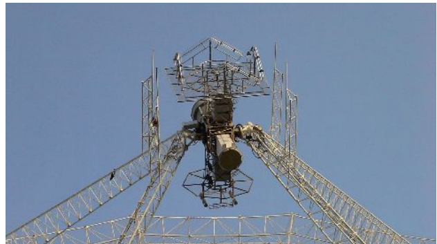
Fig. 3. Low Frequency Feed in boxing ring configuration co-located with the existing 327 MHz GMRT feed with extended reflector. The picture to the right shows its mounting on the turret of a GMRT antenna.
