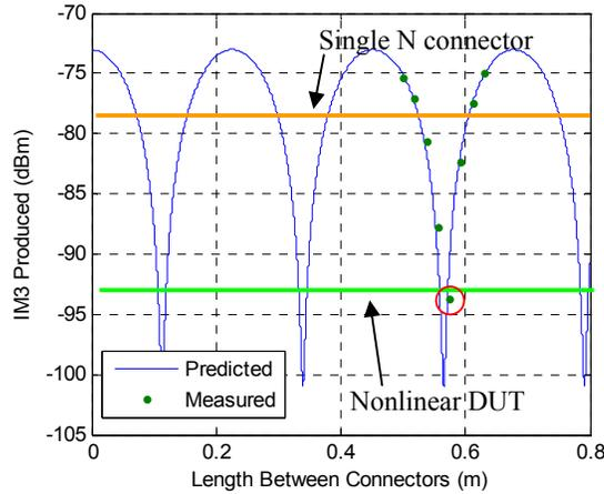
Fig. 1 Differing levels of IM produced by varying the spacing between 2 PIM-producing coaxial connectors. The orange bar shows the PIM level of the connectors individually. The green bar shows the target PIM level of the DUT at -93 dBm
