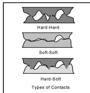
Fig. 2. Illustration of the three different types of metal contacts, showing how hard-soft contacts maximize both film penetration and contact area.
