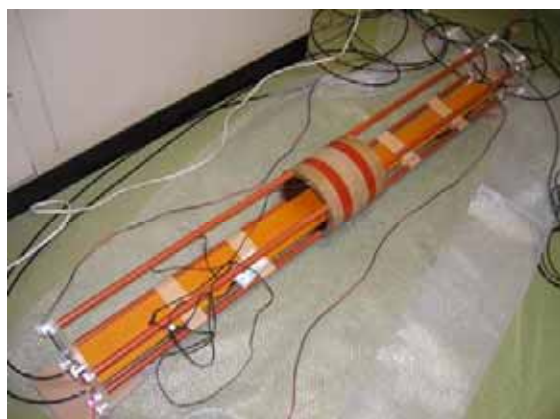
Helmholtz' coil for complex exposure of DC and ELF magnetic fields
