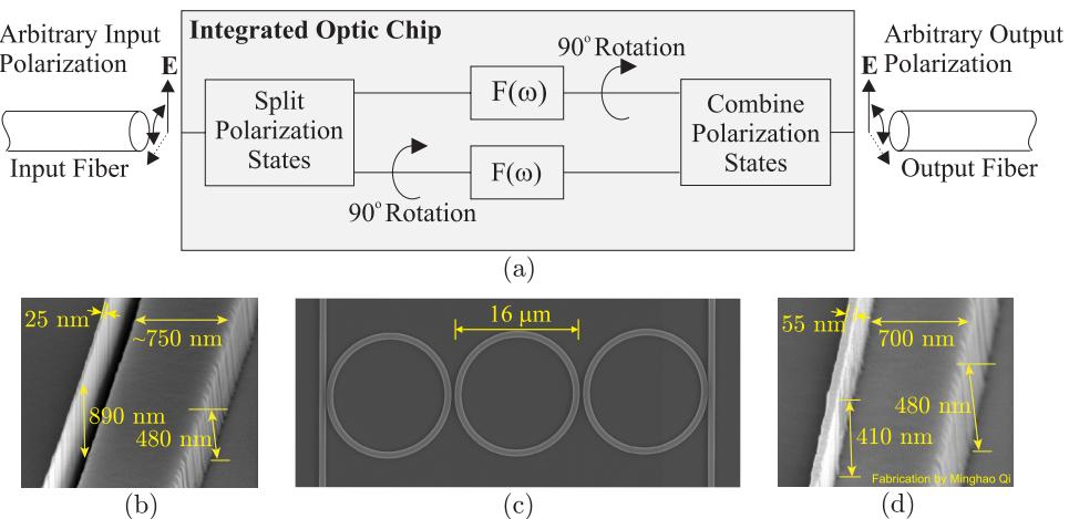
Fig. 1 (a) Diagram of an integrated polarization diversity scheme along with scanning electron micrographs of (b) an integrated optic polarization splitter, (c) micro-ring resonator, and (d) an integrated optic polarization rotator.
