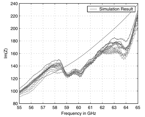
Figure 9: Measurement and simulation result of the impedance at the diode feed point, simulation result obtained using FEKO
