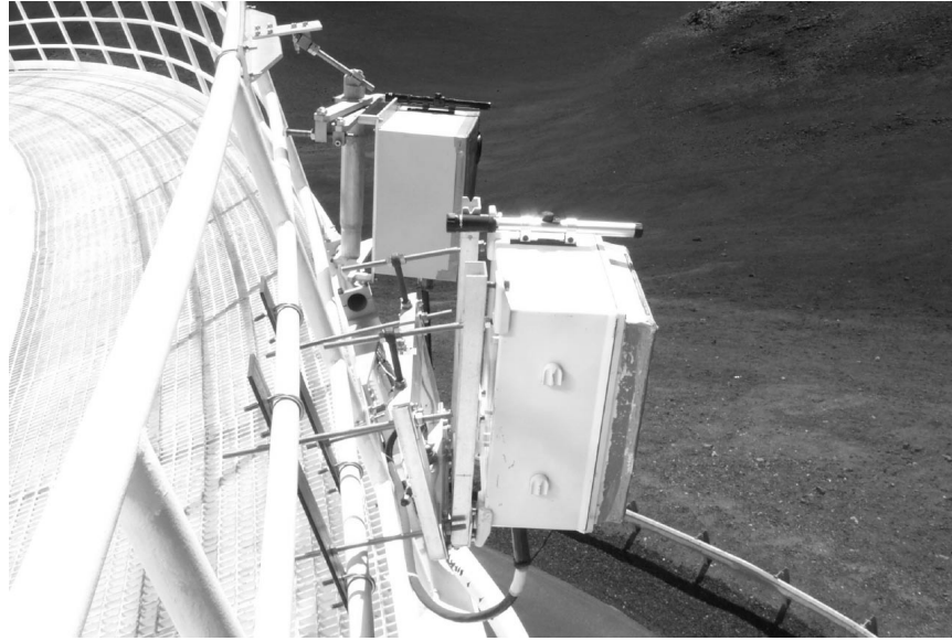
Figure 2: Test signal sources emitting phase-locked tones at 232.4 & 682.5 GHz, mounted on the cat-walk of the Subaru Telescope.
