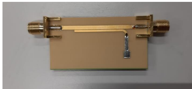
Figure 1. Humidity transducer based on a bimorph paper-aluminum cantilever [3].
