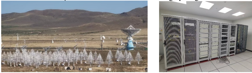
Figure 1. The antennas (left) and the indoor receivers (right) of the new radio heliograph, the compact array used for calibration is also shown at the bottom of the left panel.
