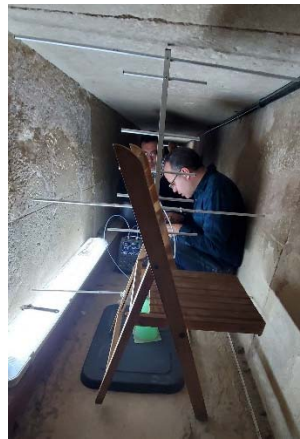
Figure 1. Yagi-Uda antenna in a horizontal corridor in the Great Pyramid.
