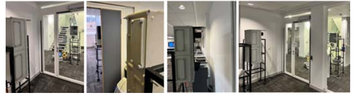
Figure 3. Setup of measurements: Glass door (first), Wooden door (second), Wall partition 1 (third), Wall partition 2 (fourth)
