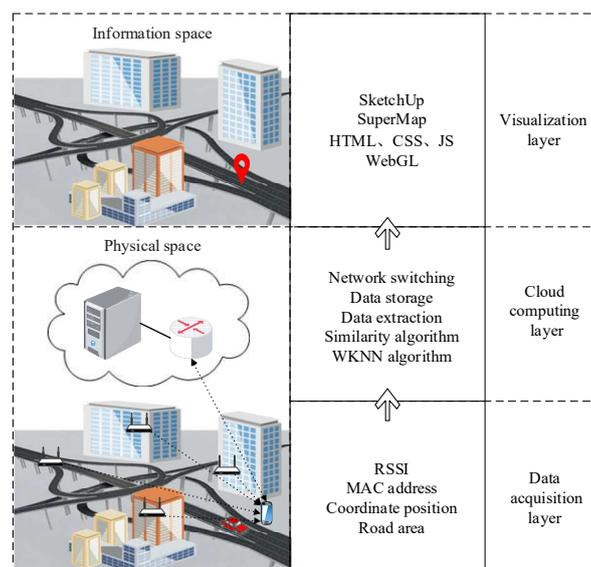
Figure 1. The system architecture of vehicle navigation model based on WiFi
