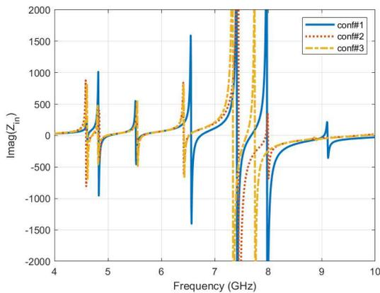
**Figure 4.** Example of variation of the resonances of the three dimensional RFID tag as a consequence of different inclusion configurations.
