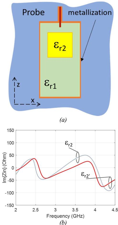
**Figure 2.** (a) Representation of the nested structure of the proposed chipless RFID tag consisting of a main hosting structure realized with a dielectric of permittivity  $\epsilon_{r1}$  and an inclusion of a different material (permittivity  $\epsilon_{r2}$ ) and (b) expected variation of the frequency response for different material inclusions.
