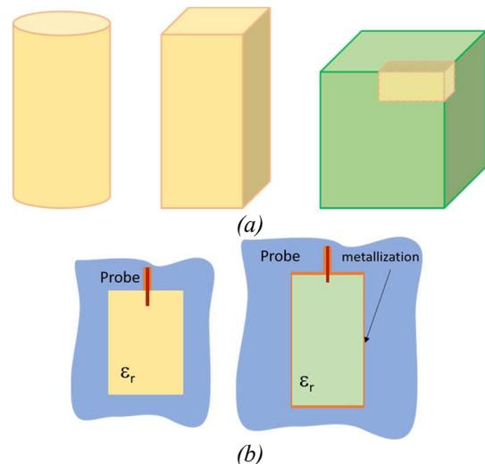
**Figure 1.** Example of different shapes and configurations of three-dimensional chipless RFID tags (a) and reading process by using a probe coupled to open/metallized resonators.
