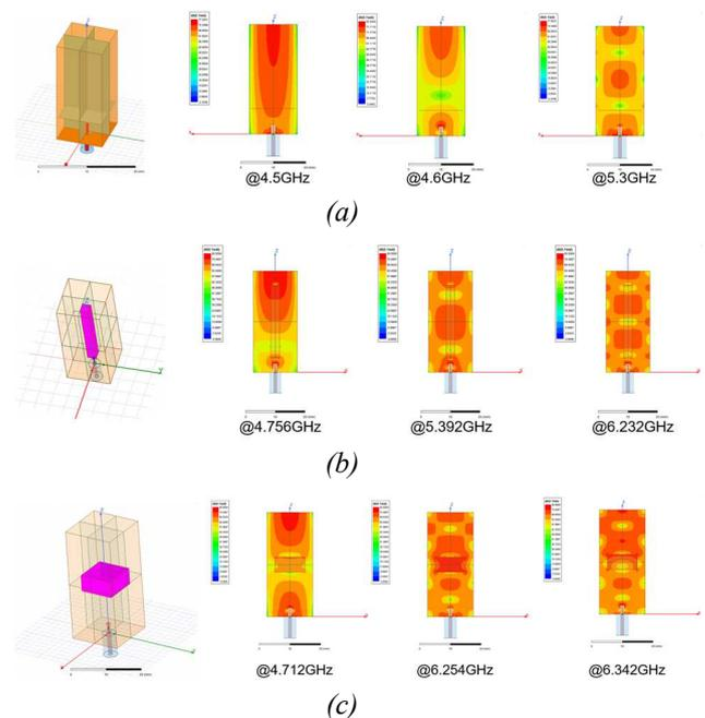
**Figure 3.** Examples of resonance frequencies variation depending on the shape and position of the inclusion: (a) no inclusion, (b) thin axial inclusion along the main axis and (c) wide inclusion located in the center part of the resonator. Three electric field distributions are reported for each case.
