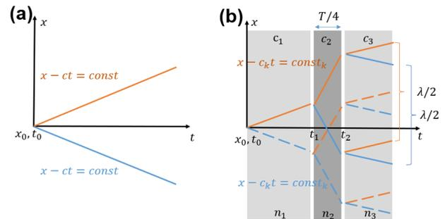
**Figure 1.** The space-time diagram with characteristic lines in (a) a time-invariant medium, and (b) a temporal system where there is an antireflection temporal coating (two temporal boundaries exist at  $t_1$  and  $t_2$ ). The orange and blue lines correspond to the forward and backward waves, respectively.
