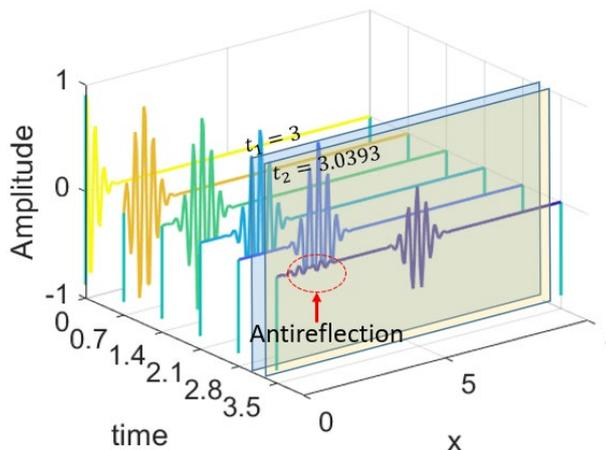
Figure 2 (a) shows the calculated distribution of the  $D$  - field as a function of time. The area marked by a red circle indicates that the reflection has indeed been canceled. The
