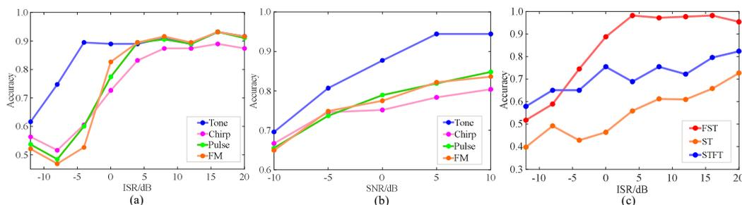
**Figure 2.** Detection accuracy of FST. (a) Average accuracy under different interference levels. (b) Average accuracy under different channel conditions. (c) The average accuracy of FST, ST and STFT with SNR=5dB.
