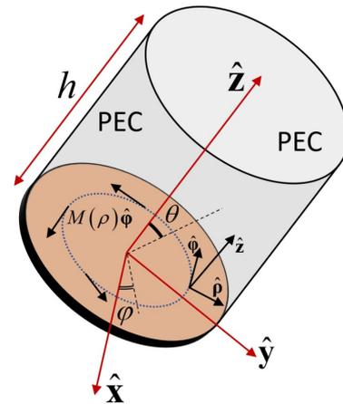
**Figure 1.** Geometry of the problem. An azimuthally-invariant magnetic current distribution shaped as a first order Bessel function radiates inside a cylindrical metallic cavity, thus exciting a specific field distribution inside it.
