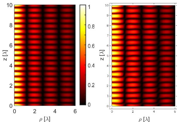
**Figure 4.** Normalized electric field longitudinal component radiated by the magnetic current distribution in (1), with  $k_{\rho a} = k \sin \theta_a$ , being  $\theta_a = 15^\circ$ , inside a metallic cylindrical cavity of radius  $b = 6\lambda$  and height  $h = 10\lambda$ . On the left (right), analytical model (simulation by COMSOL Multiphysics).
