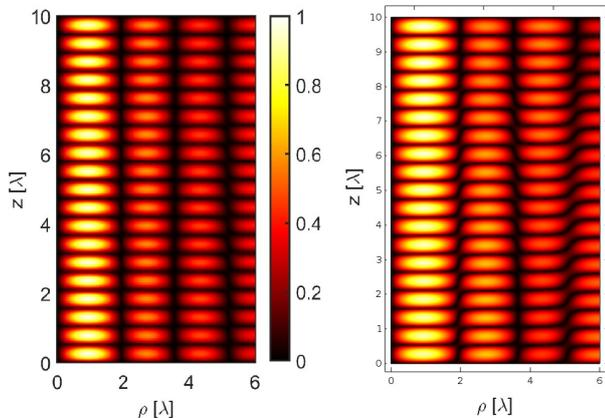
**Figure 3.** Normalized electric field radial component radiated by the magnetic current distribution in (1), with  $k_{\rho a} = k \sin \theta_a$ , being  $\theta_a = 15^\circ$ , inside a metallic cylindrical cavity of radius  $b = 6\lambda$  and height  $h = 10\lambda$ . On the left (right), analytical model (simulation by COMSOL Multiphysics).
