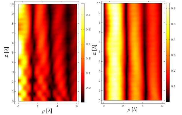
**Figure 2.** Electric field components (longitudinal, on the left; transverse, on the right) radiated in free-space by the magnetic current distribution in (1), with  $k_{\rho a} = k \sin \theta_a$ , being  $\theta_a = 15^\circ$ . Such a field distribution resembles that of a longitudinally-polarized limited-diffractive Bessel beam, as proven in [4, 5].
