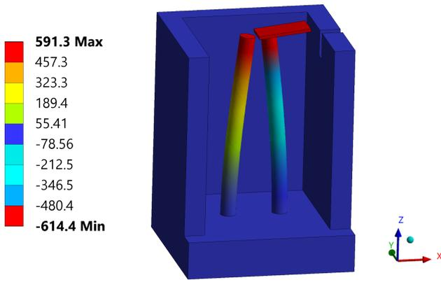
**Figure 5.** Figure depicts the mechanical activity of the implant at x-direction.
