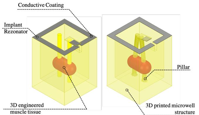
**Figure 1.** Figure depicts the components of the designed implant and muscle actuation.
