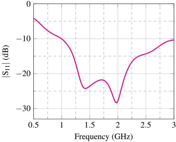
**Figure 3.** Reflection coefficient of the reader antennas.
