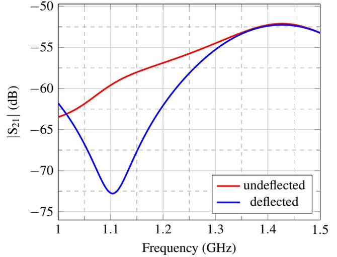
**Figure 7.** The change in the transmission behavior between the reader antennas in dBs, vs. frequency
