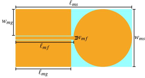
**Figure 2.** Antenna model and the parameterized dimensions.
