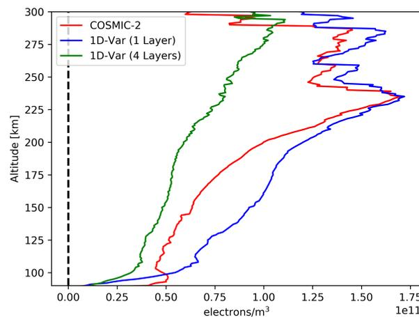
**Figure 1.** Root mean square error (RMSE) altitude profiles for COSMIC-2 and the 1D-Var retrieval with only an F2 layer (blue) and F2+F1+E+Topside layers (green) compared to ionosonde observations.
