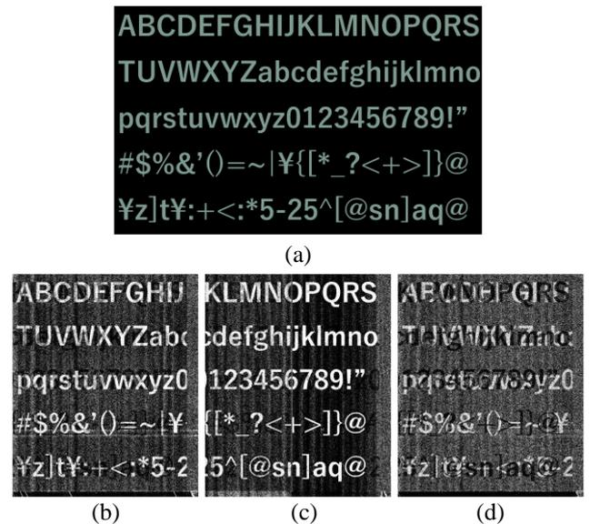
**Figure 6.** (a) The image displayed on the laptop PC. Reconstruct video images at the center frequency of (b) 303 MHz, (c) 454 MHz, (d) 604 MHz.
