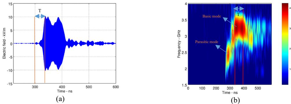
**Figure 1:** (a) Filtered signal (b) Gabor transform of the measured signal
