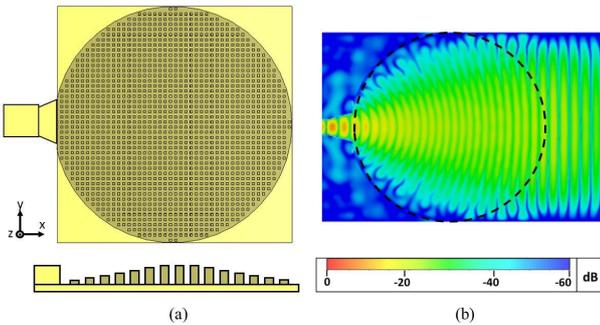
**Figure 2.** (a) Top view (top) and cross section (bottom) of the Luneburg lens fed by horn antenna. (b) Electric field
