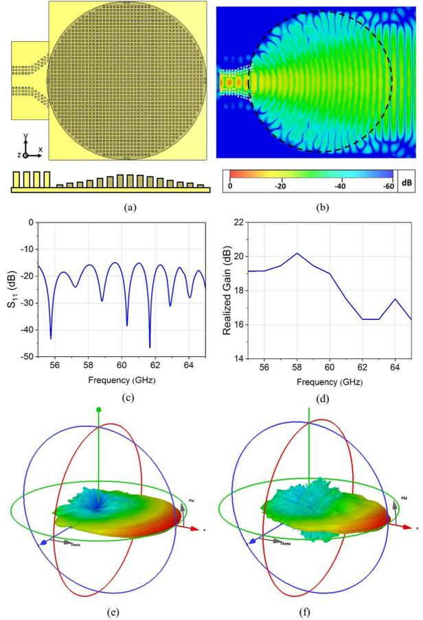
**Figure 3.** (a) Top view (top) and cross section (bottom) of the Luneburg lens fed by a GGW horn antenna. (b) Normalized electric field magnitude  $|\text{Re}\{E_z\}|$  at 58 GHz in decibel scale. Simulated results of the structure. (c) Magnitude of the reflection coefficient in dB. (d) Peak realized gain vs frequency. Radiation patterns of (c) Luneburg lens fed by horn antenna and (d) Luneburg lens fed by GGW horn antenna.
