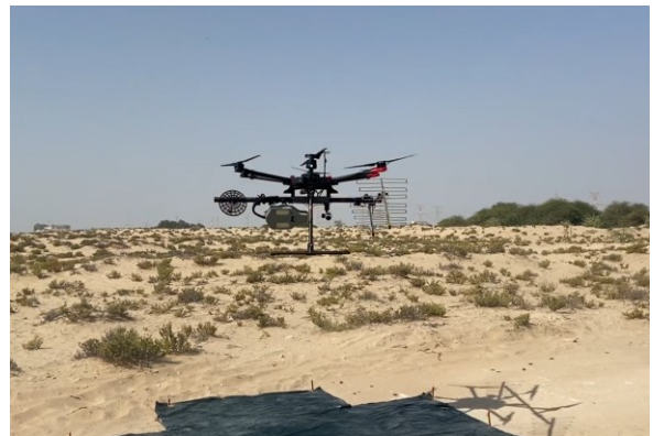
Figure 1. Drone-borne SAR system in the survey area.
