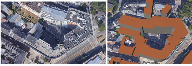
Figure 2. 3D view of an existing site (left), numerical model with buildings and fixed antenna locations (right)
