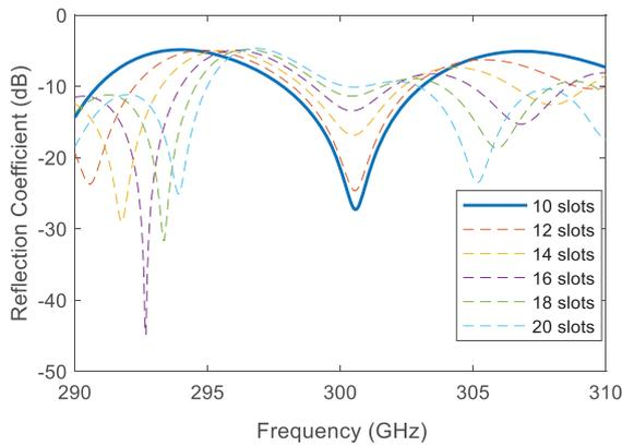
**Figure 2.** Simulated reflection coefficients of the antenna for varying numbers of radiation slots.
