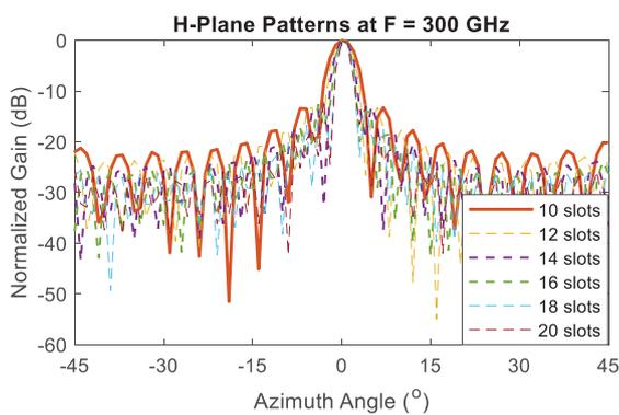
**Figure 3.** Simulated normalized radiation patterns at F = 300 GHz for various radiation slots.
