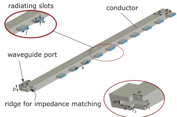
**Figure 1.** Basic structure of the proposed slotted waveguide antenna for THz applications.
