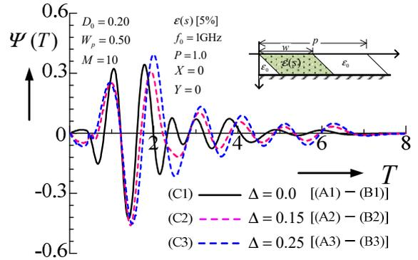
**Figure 6.** Differential waveform  $\Psi(T)$  of the electric and magnetic fields for varying slanted widths.  $\Psi(T)$  is the result of  $E_z^{(r)}(T) - H_y^{(r)}(T)$ .
