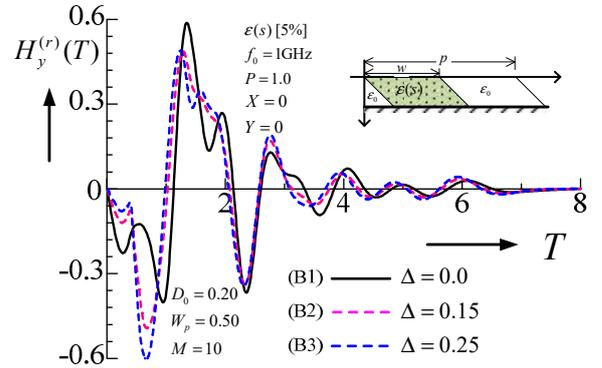
**Figure 5.** Waveform of reflected magnetic field for varying normalized slanted width.
