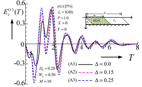
**Figure 4.** Waveform of reflected electric field for varying normalized slanted width.
