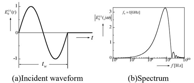
**Figure 2.** Incident pulse waveform and its spectrum (a)incident waveform, (b)spectrum.
