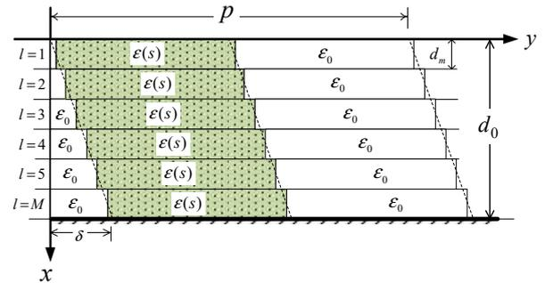
**Figure 3.** Example of multilayer division in one period for case of  $M = 6$ .
