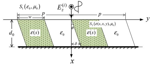
**Figure 1.** Structure and coordinate system for slanted grating formed by periodically arrayed dispersion medium and slanted air region.
