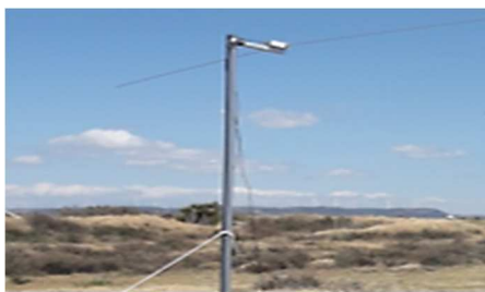
Figure 8. The active array under test installed on a temporary mast.
