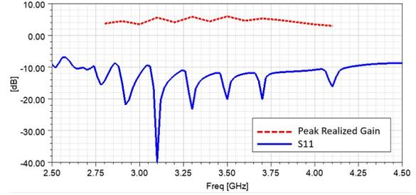
**Figure 2.** Reflection coefficient and peak realized gain of the antenna. [12]
