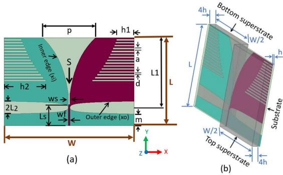
**Figure 1.** Miniaturized antipodal Vivaldi antenna- (a) top view, (b) isometric view; (parameters:  $L = 30.2$  mm,  $W = 44.4$  mm,  $a = d = 0.5$  mm,  $h1 = 6$  mm,  $h2 = 14.27$  mm,  $L1 = 24$  mm,  $L2 = 2.2$  mm,  $p = 18$  mm,  $wf = 0.5$  mm,  $m = 4$  mm,  $Ls = 7.2$  mm,  $ws = 0.5$  mm,  $h = 0.64$  mm). [12]
