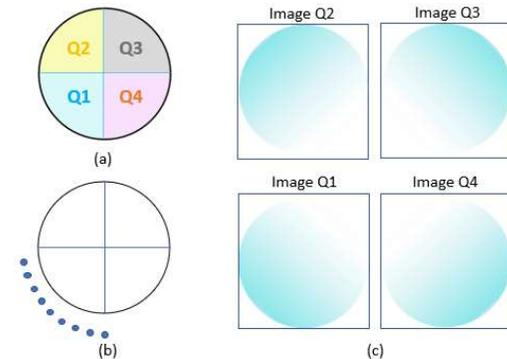
**Figure 3.** Microwave head imaging system: (a) division of a head plane into four quarters, (b) antenna positions in front of the first quarter, (c) focusing region in the image obtained by scanning through each quarter. [12]
