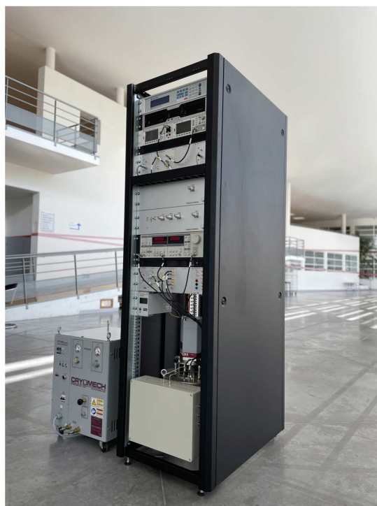
Figure 1. ULISS-2G CSO. The cryostat is integrated at the bottom of the 19" rack. On the left, the 3 kW water cooled He compressor. This unit is equipped with a 9,192 MHz synthesizer and can serve as a local oscillator for a cesium cold atoms fountain.
