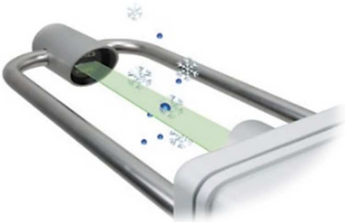
Figure 4. Conceptual scheme of the measurement of size and terminal velocity of drops with a laser disdrometer. Drop size and velocity are derived from the obstruction of the infrared laser beam (green area).
