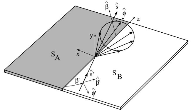
**Figure 1.** Geometry relevant to the plane wave diffraction by the junction between co-planar resistive half-planes.
