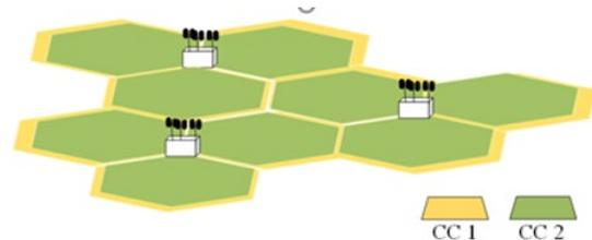
**Figure 1.** Carrier Aggregation Deployment in the same Macrocell.
