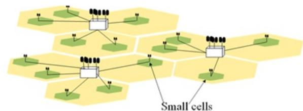
**Figure 2.** Carrier Aggregation Deployment between Macrocell and Small Cell.
