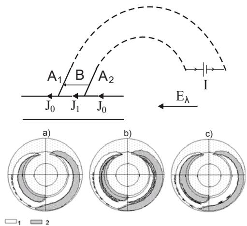
**Figure 2.** Ionosphere-magnetosphere coupling. Field-aligned currents generated in the magnetosphere: 1 - zone of inflow currents, 2 - zone of outflow currents; a)  $t=0$  s; b)  $t=1000$  s; c)  $t=2800$  s
