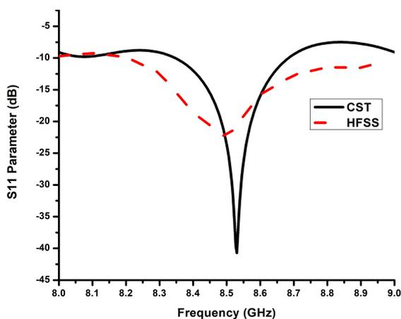
**Figure 3.** Comparison of  $S_{11}$  Parameters of DRA in HFSS and CST solvers
