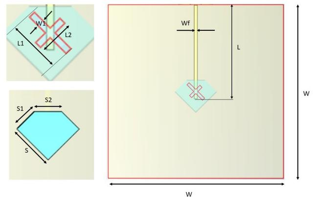
**Figure 1.** Geometry of the Antenna
