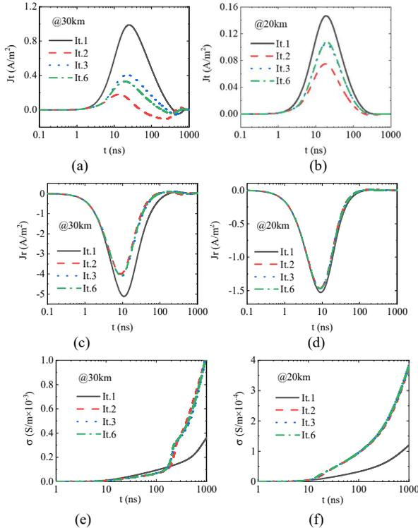
Fig. 4 Numerical results simulated by the proposed iterative scheme of transverse Compton current at heights of 30 and 20 km (a and b), radial Compton current at heights of 30 and 20 km (c and d), and air conductivity at heights of 30 and 20 km (e and f), the total prompt gamma dose was 3 kT.
