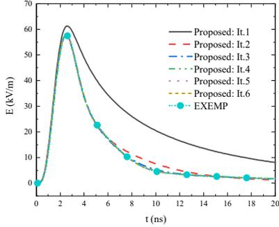
Fig. 3. Numerical results of the electric field (on the ground) time-domain waveform, simulated by the EXEMP method and the proposed iterative scheme.
