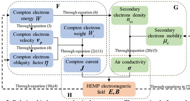
Fig. 2. Relationship between physical parameters. The equation before and after the slash are used in the case with and without the consideration of self-consistency, respectively.
