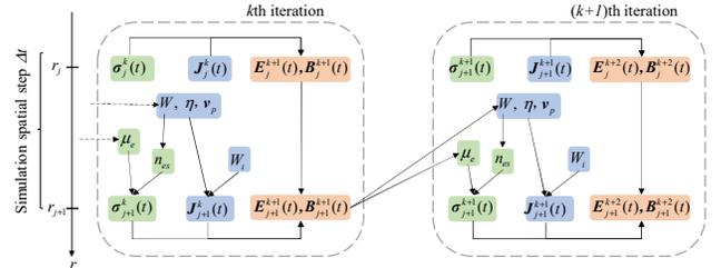
Fig. 1. Graphical depiction of the computation order of the HEMP physical parameters in the proposed iteration scheme with the consideration of self-consistency.
