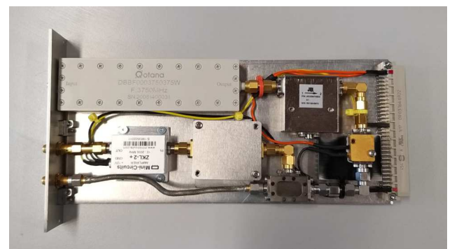
Figure 5: assembled RF down converting board
