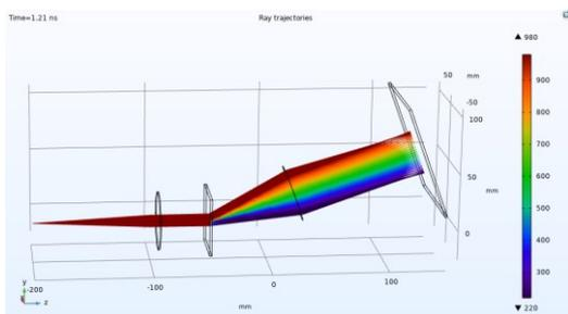
**Figure 4.** Transmission-based grating model of the spectrometer.
