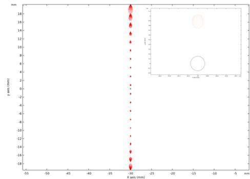
**Figure 5.** Spot diagram at the target plane of the detector (CCD). A closer view of the beam spot at the target plane is shown in the inset. The black circle with 300  $\mu\text{m}$  diameter is shown in both figures for reference.
