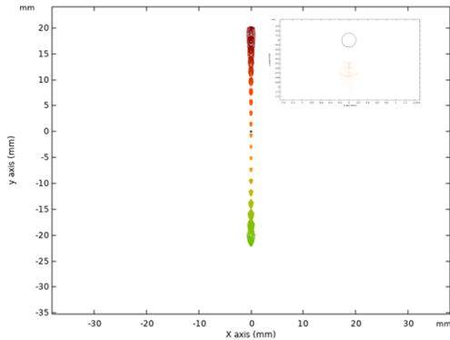
**Figure 7.** The spot diagram of the reflection-based grating model on the detector plane. The inset shows a circle with 300  $\mu\text{m}$  diameter for reference.
