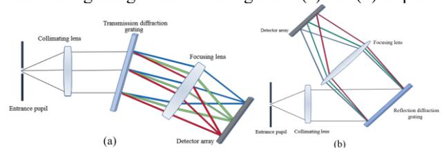
**Figure 1.** Schematic of a simplified spectrometer with a transmission-based diffraction grating (a) and a reflection-based diffraction grating (b).
