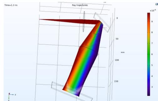
**Figure 6.** Reflection-based grating model of the spectrometer.
