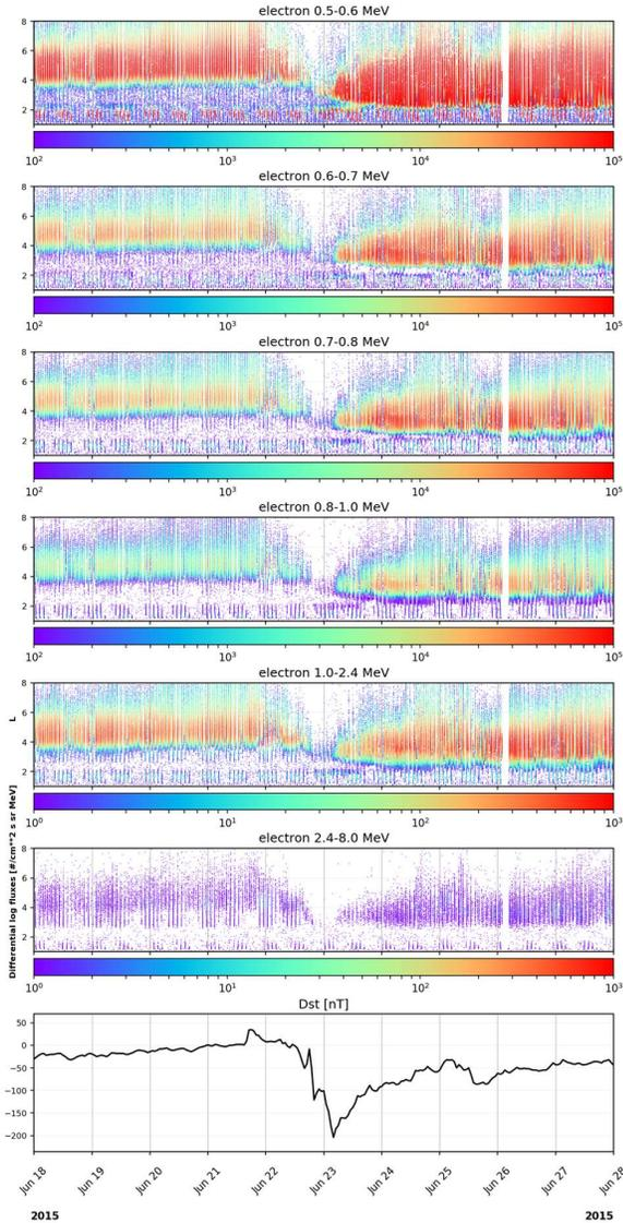
**Figure 1.** Electron fluxes observed by EPT from 18 June 2015 up to 28 June 2015, as a function of the McIlwain parameter  $L$  (vertical axis) and time (horizontal axis) for the 6 electron energy channels. The observed Dst (Disturbed Storm Time) index is given in the bottom panel.
