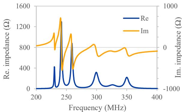
**Figure 4:** Impedance (real and imaginary part) of the final resonator with 1.52 mm wide endrings
