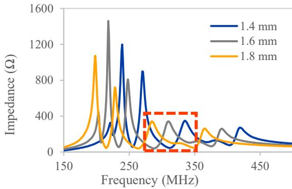
**Figure 3:** Comparison of the resonators with different width of the endrings
