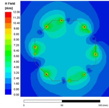
**Figure 5:** Magnetic field distribution in the half of the width of the resonator (top view)
