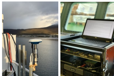
Figure 1. Antenna and scintillation recorder onboard of the Polarstern vessel [3]
