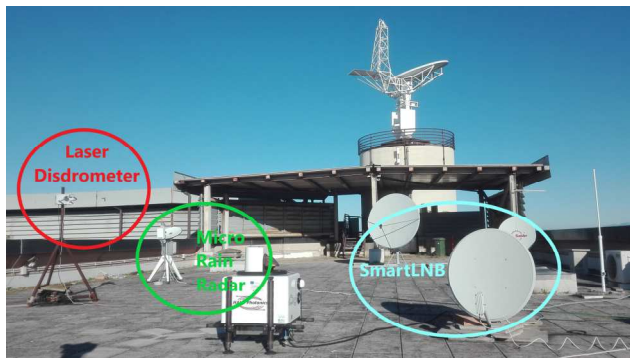
Figure 1: Experimental set-up on the roof of ISAC-CNR in Rome. Circled are the instruments involved in the experiment.
