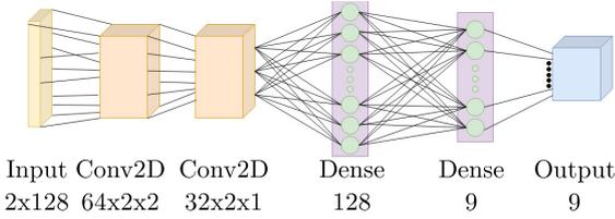
**Figure 1.** Simplified structure of the used CNN
