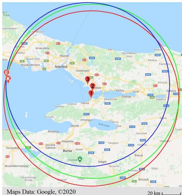
Figure 4. Trilateration result of offshore Marmara earthquake. Locations labeled as 1, 2 and 3 are selected sensing nodes in FOC, E is estimated earthquake epicenter location and K is the earthquake epicenter location provided by KOERI.
