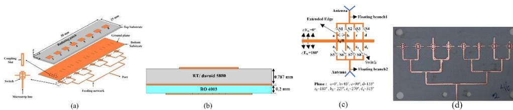
**Figure 1.** a) Structure of the antenna array b) Side view) 3-bit phase shifter d) Fabricated antenna
