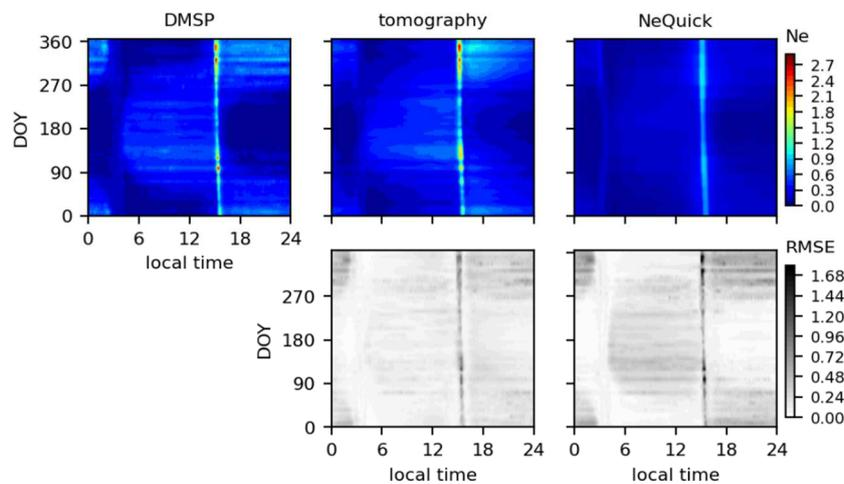
**Figure 1.** Electron density and root mean square error in 2013 for the in-situ data (DMSP), NeQuick and the developed approach (tomography). The electron density Ne ( $\text{el}/\text{m}^3$ ) was estimated with daily averages.
