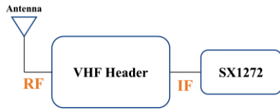
Figure 1: Block Diagram of the system. The VHF header transmits/receives RF to/from the antenna. VHF header also transmits/receives IF to/from the SX1272 module. VHF header converts RF into IF, and IF into RF.
