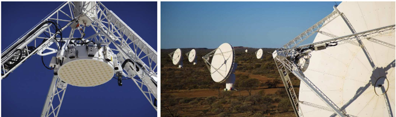
Figure 1. The Australian SKA Pathfinder (ASKAP) is a powerful radio interferometer which consists of 36 x 12-m dishes, forming a 6-km diameter array. Each ASKAP antenna is equipped with a wide-field Phased Array Feed (PAF) allowing to form 36 beams that together provide a typical field of view of 30 square degree. See Hotan et al. (2021) for more details.
