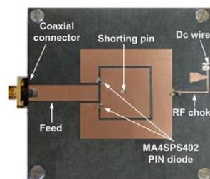
**Figure 1.** A picture of the fabricated prototype of the V2X printed antenna with switchable broadside and conical radiation patterns.
