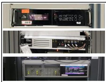
**Figure 1.** NavIC receiver, GNSS receiver and TWSTFT modem operational at PTF
