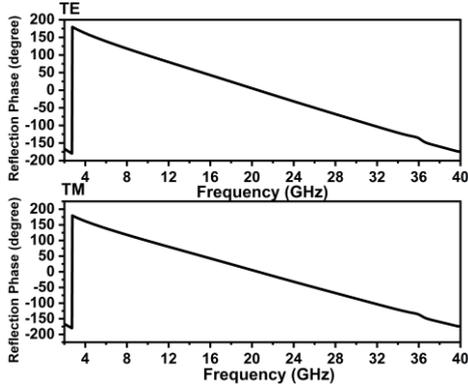
**Figure 5.** Phase of reflection coefficient ( $S_{11}$ ) of FSS in TE and TM planes of polarization.
