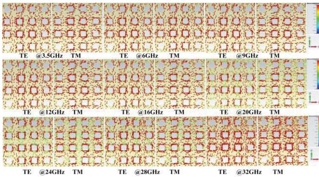
**Figure 6.** Simulated surface current on FSS unit cell for both TE and TM planes of polarization at different frequencies, covering the entire FSS bandwidth.
