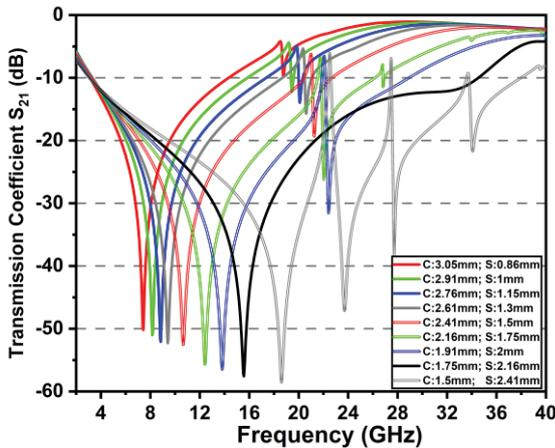
**Figure 3.** Transmission ( $S_{21}$ ) and reflection ( $S_{11}$ ) coefficients of FSS for different values of  $s$  &  $c$ .
