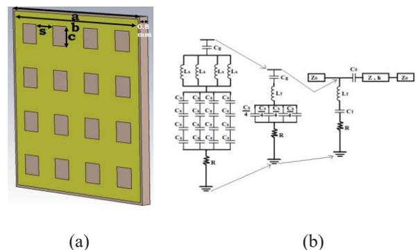
Figure 1. (a) Schematic of FSS unit cell with design parameters (b) Equivalent circuit model of FSS
