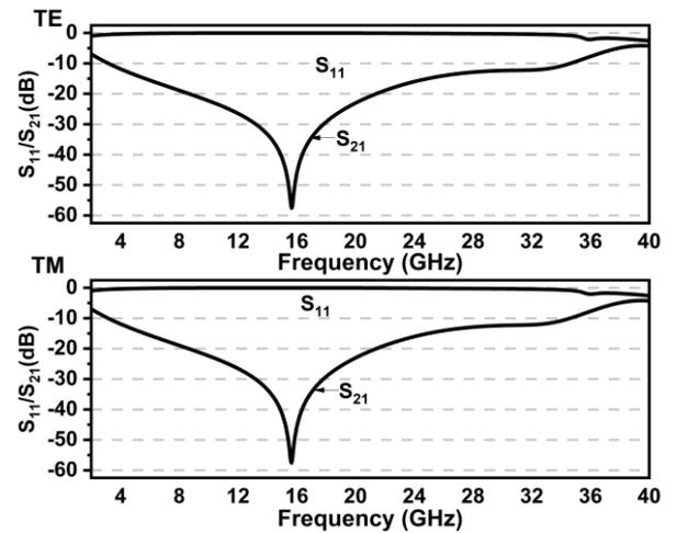
**Figure 4.** Transmission ( $S_{21}$ ) and reflection ( $S_{11}$ ) coefficients of FSS in TE and TM planes of polarization.
