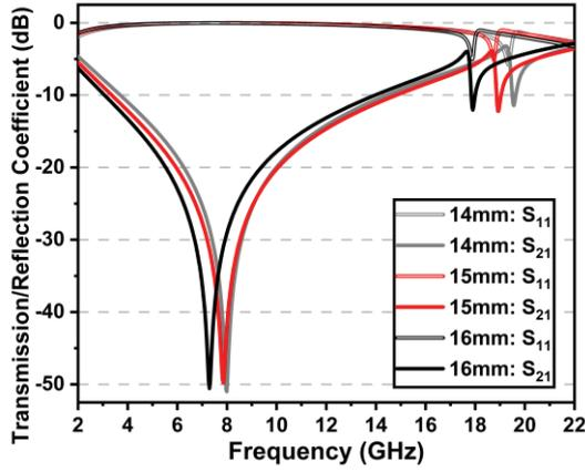
**Figure 2.** Transmission ( $S_{21}$ ) and reflection ( $S_{11}$ ) coefficients of FSS for three different values of unit cell outer dimension (a).
