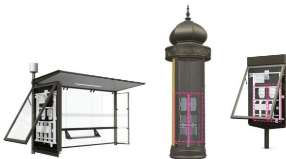
Figure 2: illustration of small cells integration in urban furniture.
