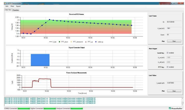
Figure 5 Data View of the control and demonstration software. Top: received RCU frames and capacitor charge state vs. time. Middle: Signal generator output vs. time. Bottom: Power analyzer measurement readings vs. time.
